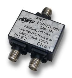
Model EWT-52-0081 is a miniature diplexer that covers the bands DC-1300 MHz and 4000-6500 MHz. The lower passband exhibits less than .50 dB insertion loss with the upper band having 1.25 dB max insertion loss. VSWR for both channels is less than 1.7:1. Channel to channel isolation is greater than 60 dB. The overall size is 1.05" x .75" x .45" with SMA connectors.
